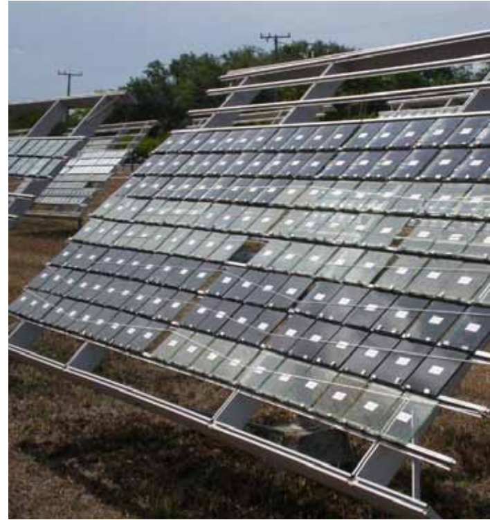
Figure 4: Exposure testing conducted in Miami, Florida, USA.
