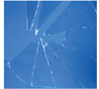
ordinary (annealed) glass breaks leaving dangerous sharp edges
