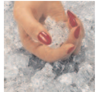
toughened (tempered) glass breaks into small, dull-edged pieces
